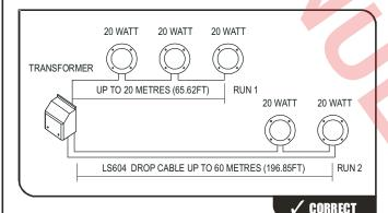
This example shows the correct way of installing the system using LS604 Drop Cable - The total load on RUN1 is 60 watts over 20 metres (65.62ft) which is allowed in the Voltage Drop Chart below (refer to (1)). The load on RUN2 is 40 watts and using a doubled cable allows the run to be up to 60 metres long (196.85ft) (refer to (2)).
