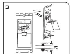
Terminate supply cable in fixture and tighten cable gland onto cable. Note: Ensure only round supply cable is used and cable gland seals on the outer insulation to ensure maximum IP rating.
