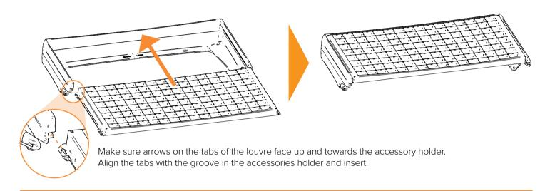
Slip the accessory holder & louver assembly over the luminaire
