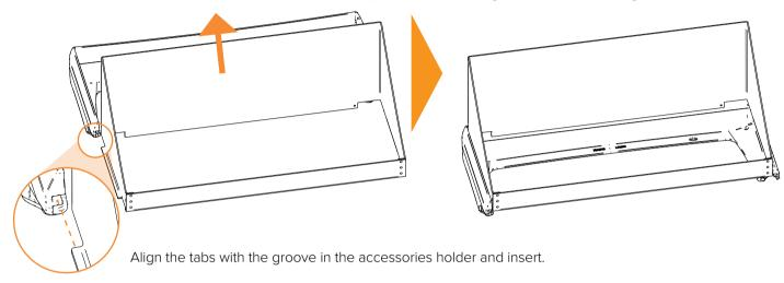
Slip the accessory holder & 45° visor assembly over the luminaire.
