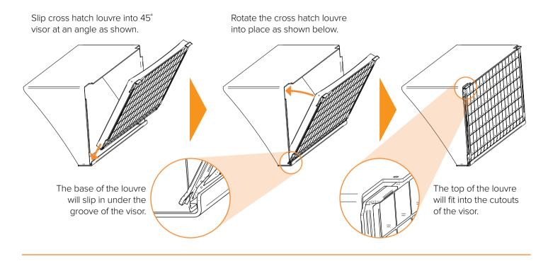
Slide 45° visor and louvre assembly into accessories holder. Make sure all the components have the right orientation and alignment as shown below.
